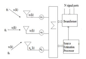
Fig.1. N element antenna array with D arriving signals
