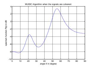
Fig.8. Simulation for MUSIC algorithm when the signals are coherent
