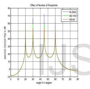
Fig.5. Simulation for effect of number of snapshots
