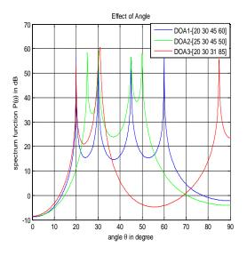
Fig.7. Simulation for Effect of Angle Spaceing
